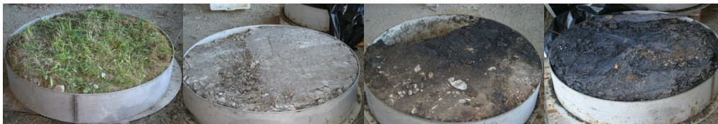
Figure 4. Freshly cut soil slices (diameter 1.13 m, thickness 20 cm), 1) topsoil 0-20cm; 2) 20-40 cm; 3) 40-60cm; 4) 60-80 cm
